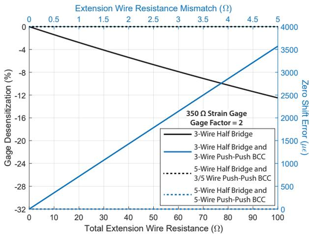
Figure 2. Strain gage desensitization and zero-shift errors
